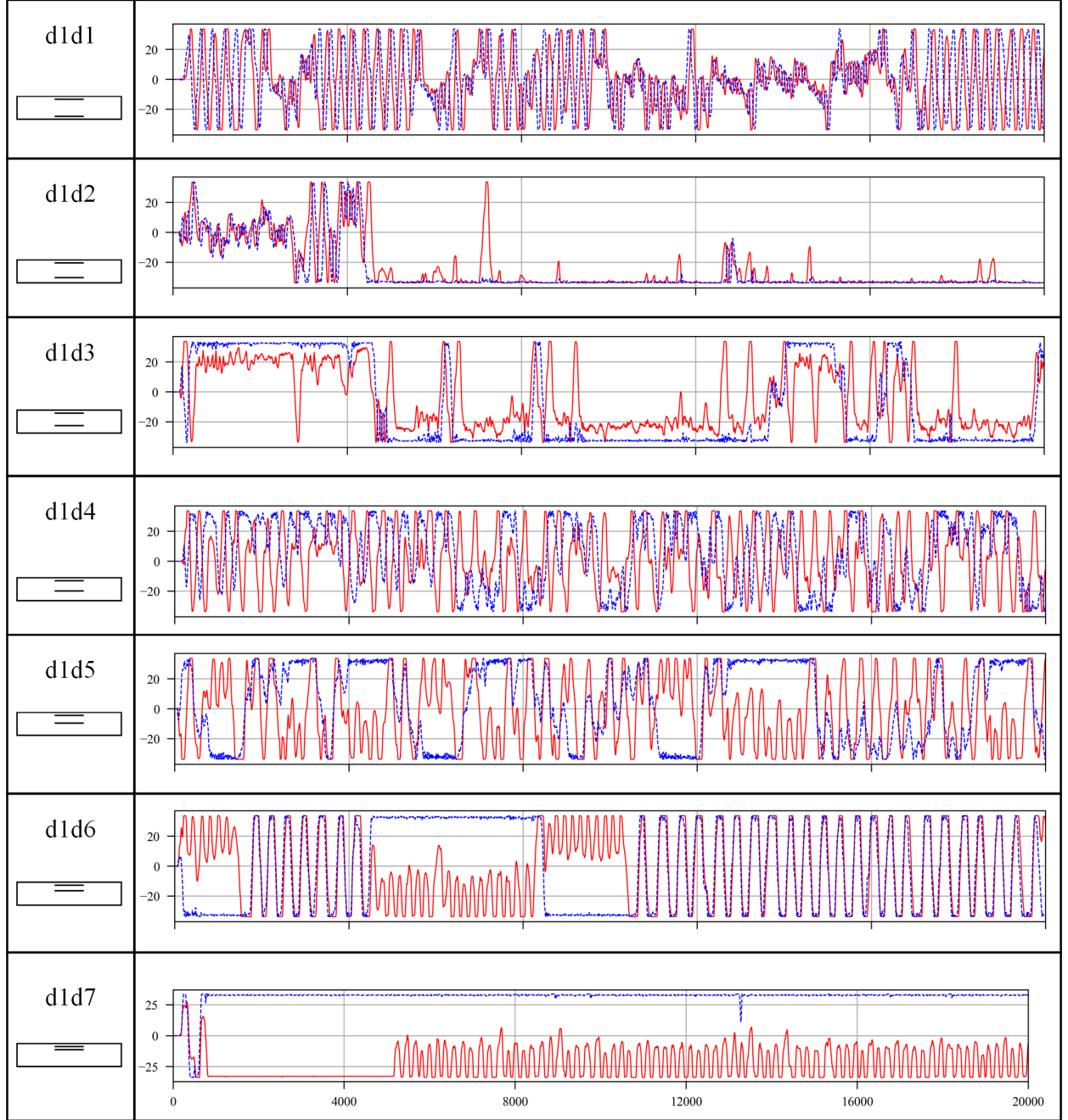
FIG. 7. The movement of the centers of the plates of size l = L/4 at Ra = 3.7 \times 10^5 for different cases, marked in each panel. The position of the lower plate is shown by blue dotted line, the position of the upper plate – by red solid line.
